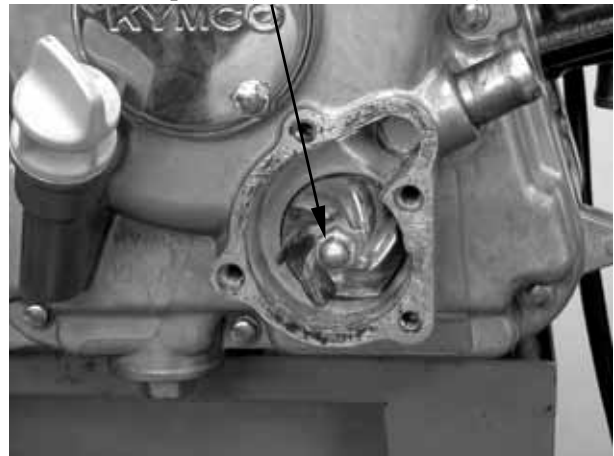
Impeller (Left Hand Threads)
